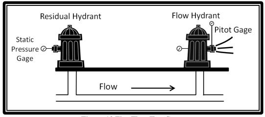
**Figure 13 Fire Flow Test Setup**
