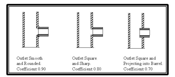
Figure 27 Hydrant Nozzle Discharge Coefficients
