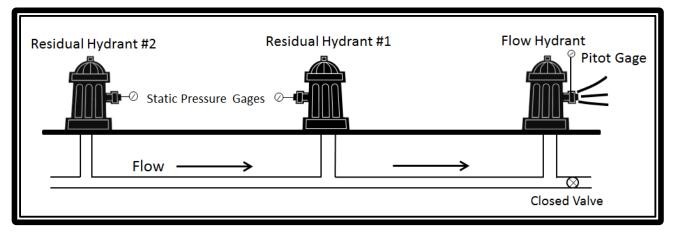
**Figure 11 C-Factor Test Setup**
