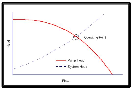
Figure 19 System Curve and Pump Curve
