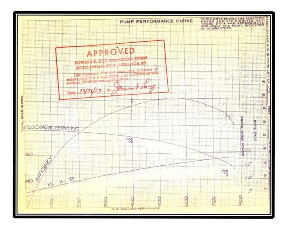
Figure 25 Manufacturer's Booster Pump Curve
