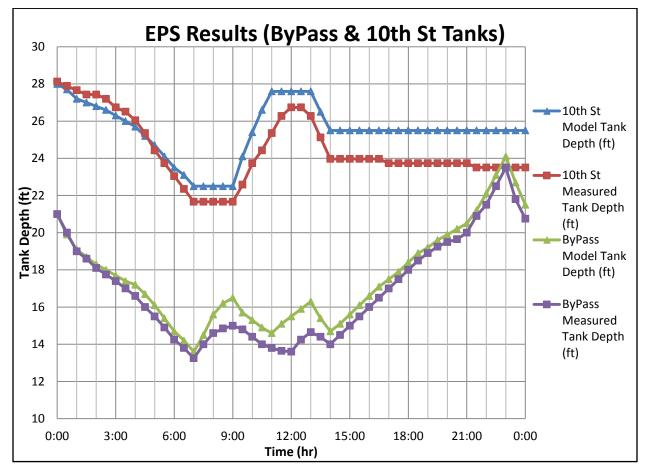
Figure 1 Summary of EPS Results for Storage Tanks for 7/3/2012
