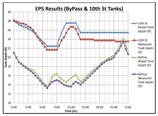
Figure 20 EPS Results for Storage Tanks for 7/3/2012
