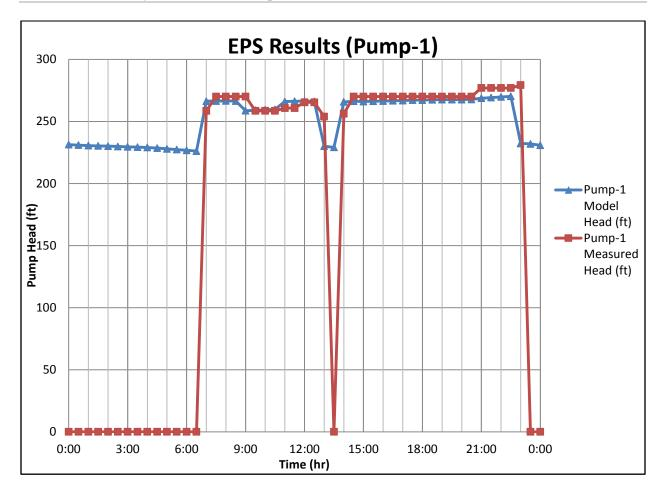
Figure 21 EPS Results for High Service Pump
